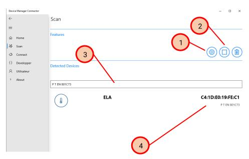
Simply click on a tag in the list to connect to that tag. The application then switches to the connection screen, which displays all the information and available commands for the selected tag.
