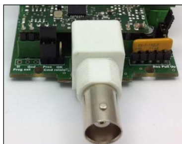
Picture: jumper J2 in PRESENCE mode
