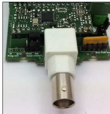
Picture: Jumper J2 in stand-alone mode
