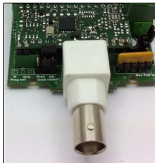
Picture: Jumper J2 in stand-alone mode
