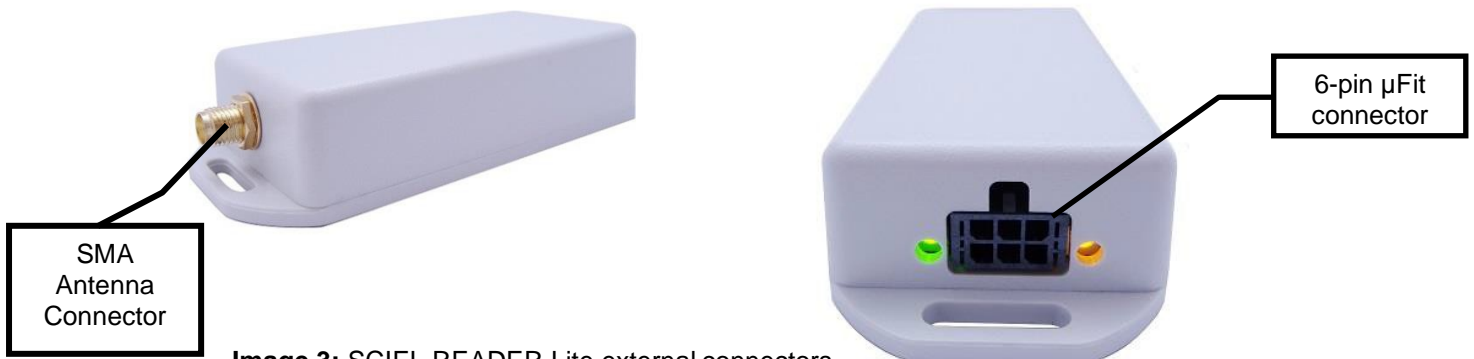
Image 3: SCIEL READER Lite external connectors
