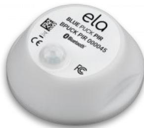
**Blue PUCK PIR** (IDF25249X) is adapted for presence or movement detection of people in a 20 cm to 5 m range (configurable) with 120° Field of View angle.
