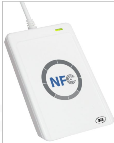
Figure3: Indicator light on NFC ACR122U reader
