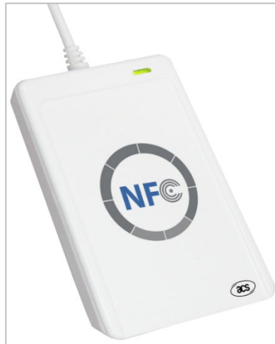
Figure3: Indicator light on NFC ACR122U reader
