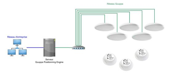
Antennas are positioned in a mesh layout, which can be more or less spread out depending on the desired localization accuracy (i.e. only presence detection, zoning, precise location).
