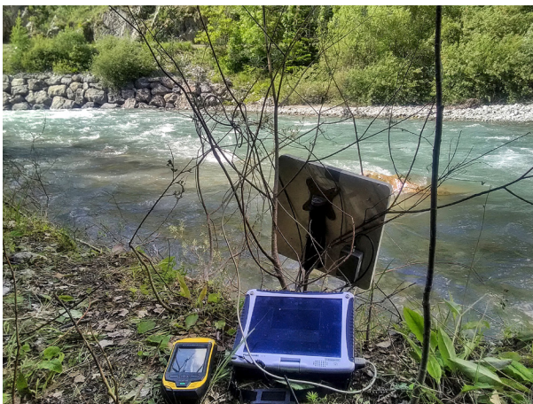
Fixed tag detection station (antenna + RFID reader)
