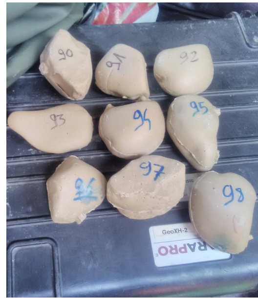
Artificial pebbles with active RFID tags
