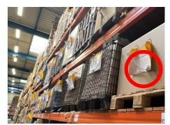
The data is then processed and analyzed by Orange Business' **IoT Smart Tracking platform**. Operators will use smartphones positioned at the entrance to each aisle to geolocate the pallet they need to within a few meters. They will also be able to **trigger the LED light** of the beacon associated with the pallet to via the mobile application, enabling them to refine their search, particularly when the pallet is stored high up.
