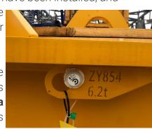
find out **in real time** on which worksite a given piece of equipment is located, as well as its utilization rate and compliance. Eventually, Potain intends to **share this inventory data** with carriers, technicians and operators **to streamline logistics operations**.
